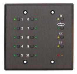
The *Rerun Architectural* is a lighting control station capable of storing up to ten 40-minute shows. Shows are recorded by capturing the output of a DMX512 console. The recorded show start and end points may be trimmed non-destructively. Each show can be set to hold the last look, loop to itself or link to another show. Shows are started by pressing one of the ten show buttons.
