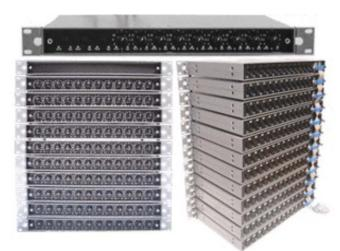
The Rotor-Router is a DMX512 distribution system featuring up to 12 inputs and an unlimited number of outputs. A system typically consists of an input module and one or more output modules. Both modules are 1.7"h x 19"w x 12"d and are normally rack mounted. A plexiglass security cover is included to prevent accidental switch changes.
