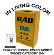
The Remote Addressing Device (model RAD) is used to set the DMX address and personality of RDM compatible products. An enhancement to DMX512 called RDM (Remote Device Management), allows users to receive status information and set parameters (such as the DMX address and personality) of compliant products using the DMX link.
