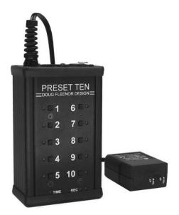
The *Preset 10 Portable* can act as a seamless backup for DMX512 lighting consoles or as a stand-alone DMX512 preset console. The *Preset 10 Portable* is capable of storing up to ten presets. These presets are recorded by capturing the output of a DMX512 console. Each preset can be assigned a unique crossfade time, from 0 to 999 seconds. Presets are recalled by pressing one of the buttons.
