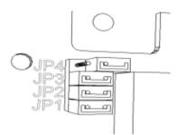
To modify a faceplate to become a REMOTE station, the shunts located at JP2 and JP4 should be removed. For safe keeping, place the shunt over only one of the pins at JP2 and JP4.
