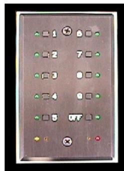
With Preset 10A installed on Starter Box
