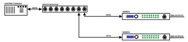
Data transport between each Art-Net or sACN capable device takes place using standard Ethernet hardware that supports multicast traffic. The diagram above utilizes a single Ethernet switch for simplicity. Any network hardware constituting a properly configured LAN may replace the Ethernet Switch blocks above.
