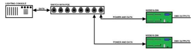
Data transport between each Art-Net or sACN capable device takes place using standard Ethernet hardware that supports multicast traffic. The diagram above utilizes a single Ethernet switch for simplicity. Any network hardware constituting a properly configured LAN may replace the Ethernet Switch blocks above.
