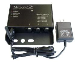
The Marconi Wireless DMX Splitter (Marconi SP) receives all 512 channels (one universe) of DMX512 using 2.4 GHz spread spectrum technology and provides three isolated DMX512 outputs.
