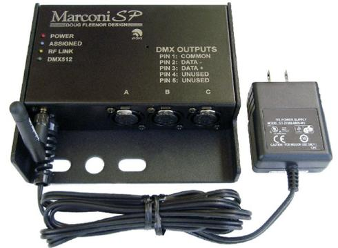
Indicators include POWER, ASSIGNED (lights when the unit is assigned to a transmitter), RF LINK (lights when the assigned transmitter is on and within range), and DMX512 (lights when DMX512 is available at the outputs). A 2 dB rubber whip antenna is standard. Gain antennas are available to increase reception range. The attached power supply operates from 100 to 240 volts AC.
