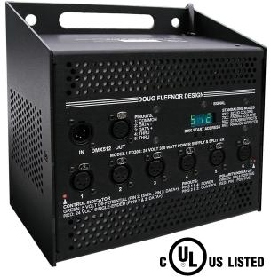
The LED300 power supply distributes DMX512 data and 24 Volt power to lighting fixtures and accessories. Primarily designed to power and control Color Kinetics ColorBlast 12 LED fixtures, the LED300 can also drive Color Kinetics iColor Cove, Altman Spectra PAR, and similar products, as well as color scrollers, gobo rotators, and other powered DMX512 controlled accessories.
