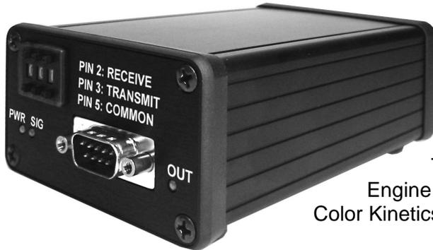
The DMX512 iPlayer 2 interface receives a DMX512 input signal and outputs RS-232 commands to the iPlayer. The interface uses three consecutive DMX512 channels: Trigger mode, Show selection, and Global intensity.
