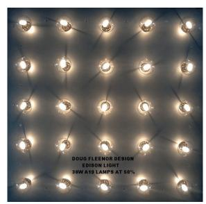
Edison is a 25 lamp fixture with 25 built-in dimmers. Lamps are spaced on six inch centers, three inches in from each edge. The 30 inch square fixture is 1 3/4 inches deep and weighs 24 pounds (without lamps). Edison is arrayable to form large, low-resolution video walls. Steel straps running down the back sides support fixtures hanging below. The front panel is solid 1/10" aluminum, free of visible hardware, and can be powder coated in a variety of colors (stock is silver).
