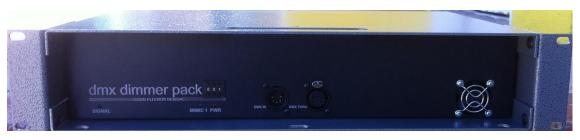
The DMX24DIM and the DMX24DIM-2U are twenty-four output dimmers designed for high efficacy loads, low idle power, and minimal losses. Typical loads include Christmas light strings (LED and incandescent), and low power lamps such as LED, neon, compact fluorescent, electronic and magnetic low voltage, halogen and incandescent. Typical applications include Christmas tree lighting, cue lights, signs, marquees, and practicals.
