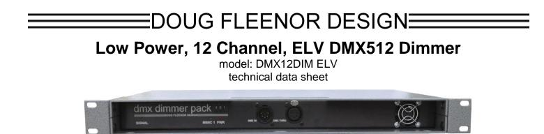
The DMX12DIM ELV is a twelve output dimmer designed for high efficacy loads, and minimal losses. This dimmer uses "reverse phase" (aka: "trailing edge") dimming techniques and MOSFET power devices. This type of control is required for proper dimming of many LED fixtures. Each output can drive loads up to 100 Watts. Each channel may be configured for reverse phase dimming (default), forward phase dimming, or non-dim operation.
