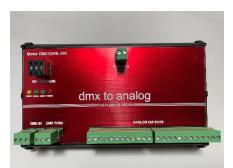
The DMX12ANL-DIN is a 12 channel DMX512 to analog 0-10V interface. It uses pluggable terminal blocks for the DMX512 in and thru connections, analog outputs, and DC power input. The device mounts on standard 35mm "top hat" DIN rail. It is powered by 12 to 24VDC. The DMX12ANL-DIN can be pre-mounted in a NEMA1 electrical enclosure (model DMX12ANL-DIN-JBOX). If a power supply is needed in the enclosure, use model DMX12ANL-DIN-JBOX-PS.
