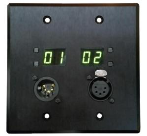
NODE2 is an Ethernet to DMX interface. The two DMX512 ports can be configured as inputs, outputs, or one of each. The standard unit is provided with two female DMX output connectors.
