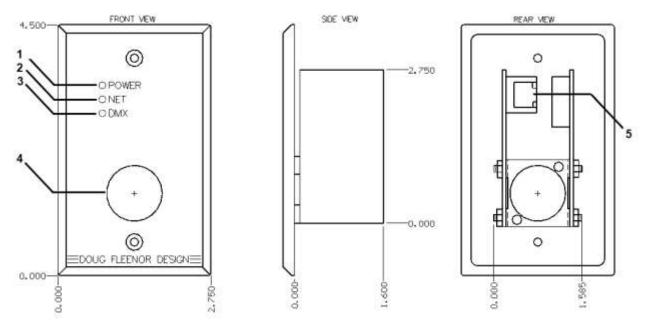
**1) POWER LED:** This indicator illuminates when the unit is powered and running. It will blink while the NODE1 is in boot loader mode.
