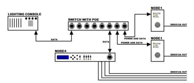
A typical network system will contain at least one console, one or more NODE1s, and an Ethernet switch. In the system shown above, the console is connected by an Ethernet cable to an Ethernet switch. An Ethernet cable is connected from the switch to each NODE1. CAT5e or higher cabling is required for 100Mbs operation in an Ethernet network.
