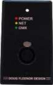
The NODE1 is a single gang wall mount Ethernet to DMX interface. It has zero boot time and accepts E1.31 sACN, draft sACN, Art-Net, Strand ShowNet, or KiNET. The single DMX port can be configured as either an input or output. Configuration is done using any web-browser (Internet Explorer, Firefox, Safari, Chrome, etc.). Powered by Power over Ethernet (PoE), the NODE1 requires only a single cat5 cable for power and signal.
