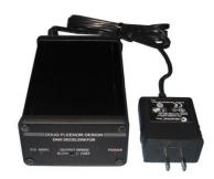
The *DMX DECELERATOR* is a DMX512 isolator and re-timing device. It can receive any signal within the DMX512 specification and it can accept some signals outside of the specification. It produces a DMX output signal with "relaxed" timing characteristics which are required by some DMX receiving devices.
