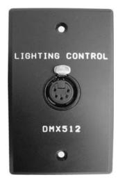
DFDNET is a buffered, optically isolated, DMX output wall plate, sized to fit a standard North American single gang electrical box. Machined from solid aluminum, the plate comes standard as black anodized with silver nomenclature. Custom colors are available on request.
