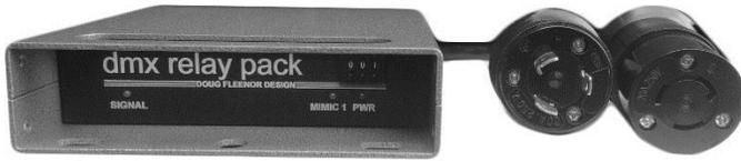
The DMX1REL20A-2POLE controls two output legs using a single channel of DMX512. The relays can switch up to a 20 amp line voltage load and are built with a 30 amp relay for robust performance. The output is suitable for 208-240VAC with both the hot legs being switched. The
