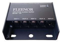
The 124 is an economical bi-directional DMX512/RDM splitter. It is available with 3 pin (model 124-3) or 5 pin (model 124-5) XLR connectors for all DMX512/RDM connections, as well as RJ45 connectors (model 124-RJ) and terminal block connectors (model 124-TB). These splitters have fully isolated inputs. The four outputs are separately driven, but are not isolated from one another.
