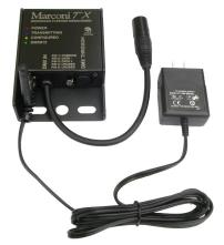
The Marconi wireless system from Doug Fleenor Design allows DMX512 distribution where cabling is not practical. Doug Fleenor believes cable is more reliable than wireless, but recognizes the advantages of wireless systems such as quicker setup, building top to building top (or cross river) communications, fewer wires to tape down, as a backup to a cable link, for troubleshooting, for focusing before the FOH cables are installed, and so on.
