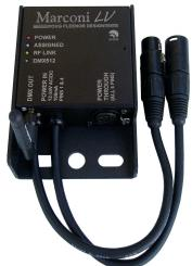
The Marconi "low voltage" (Marconi LV) is identical in performance to the Marconi SP but is powered by low voltage instead of line voltage and has only one DMX512 output. The LV is designed to mount to our LED300 power supply but can be used with any 24V system that provides power on pins 1 and 4 of a four pin XLR (color scroller for example). The LV may also be powered by an optional external supply.
